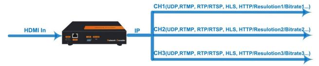
Multiple (up to 3) streams out with different protocol/resolution/bitrate...
