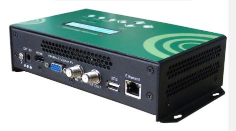
A device that allows audio and video signal input in TV distributions and video recorded and playback from a **USB** port, with applications in home entertainment, Digital Signage for hotels, shops, restaurants etc...
